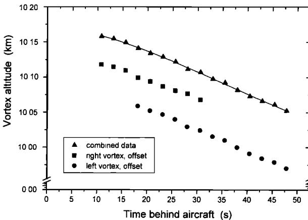
**Figure 7.** Ground-based lidar measurement of the descent of the pair of trailing vortices behind a B-747-400 aircraft, by 16 subsequent lidar profiles (same contrail as in Figure 1). Altitudes of the right and left wingtip vortex, respectively, were obtained subsequently with some overlap. The combined data points are connected by a third-order polynomial fit.
