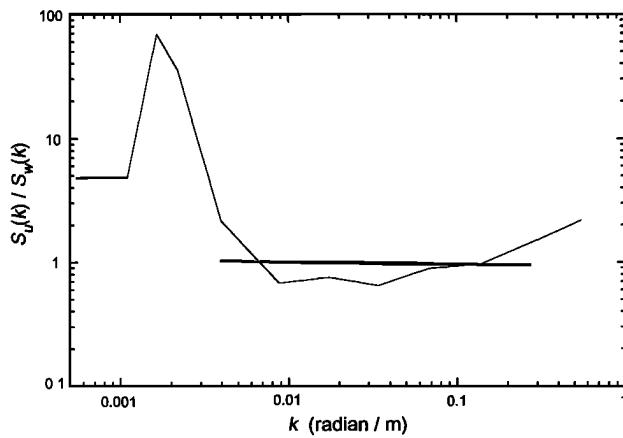
**Figure 4.** Ratio of the spectral density functions of horizontal ( $S_u$ ) and vertical velocity fluctuations ( $S_w$ ) over wavenumber  $k$  measured during a 1 min flight segment of the research aircraft FALCON at the altitude of the lidar-measured contrail (Plate 1a) and nearly coincident in time and geographical location to the lidar measurement. A wavenumber range with locally isotropic turbulence is found, as indicated by the fitted line.
