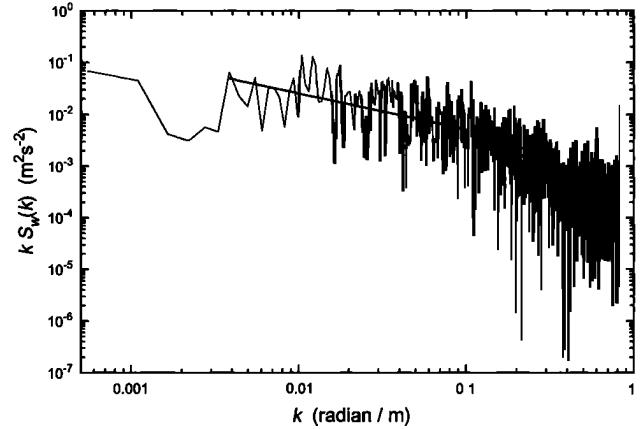
**Figure 5.** Spectral density function  $M(k) = kS_w(k)$  of vertical velocity fluctuations over wavenumber  $k$  measured during a 1 min flight segment of the research aircraft FALCON at the altitude of the lidar-measured contrail (Plate 1a) and nearly coincident in time and geographical location to the lidar measurement (same flight segment as in Figure 4).
