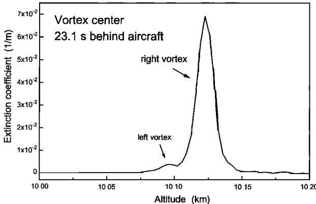
**Figure 6.** Extinction profile derived from a lidar backscatter profile (average of 10 laser pulses) penetrating one vortex wake of a B-747-400 through its center 23.1 s behind aircraft (same contrail as in Figure 1).
