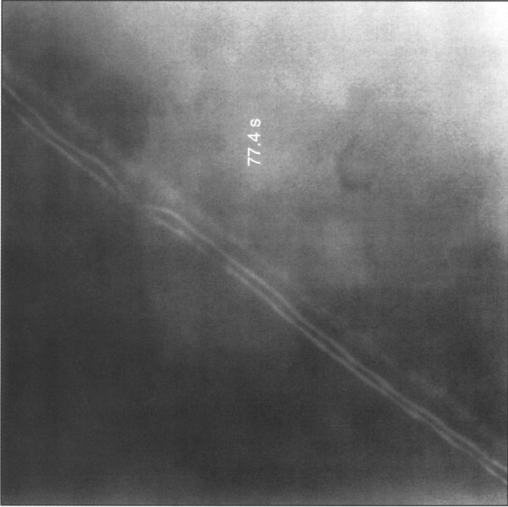
**Figure 1.** CCD image of the contrail of the B-747-400 aircraft investigated in this work (77.4 s behind aircraft). Note the “secondary-wake phenomenon,” i.e., a diffuse third plume above the pair of wingtip vortices.
