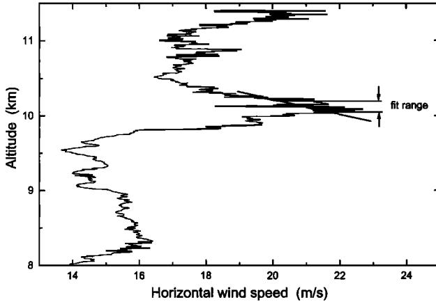
**Figure 3.** Vertical distribution of total wind speed measured during an ascent of the research aircraft FALCON nearly coincident in time and geographical location to the lidar measurement of Plate 1. The vertical fit range corresponds to the extension of the vortex phase wakes (Plate 1a). A vertical shear of total wind speed of  $dS/dz = -0.01 \pm 0.004 \text{ s}^{-1}$  is found.
