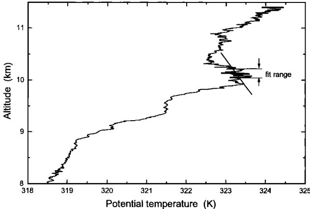
**Figure 2.** Vertical distribution of potential temperature measured during an ascent of the research aircraft FALCON nearly coincident in time and geographical location to the lidar measurement of Plate 1. The vertical fit range indicated corresponds to the vertical extension of the vortex phase wakes (Plate 1a). A vertical gradient of potential temperature of  $d\Theta/dz = -0.001 \pm 0.0008 \text{ K/m}$  is found.
