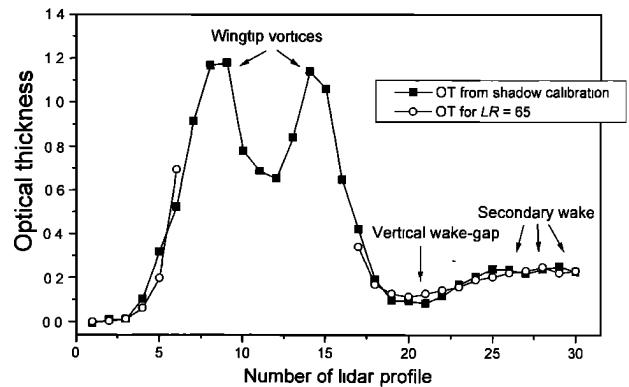
**Figure 8.** Optical thickness of the contrail of a B-747-400 along 30 subsequent lidar profiles recorded in the time period of 5.7–77.4 s behind aircraft with lidar zenith angles ranging between  $54.4^\circ$  and  $57.3^\circ$  (same contrail as in Figure 1).
