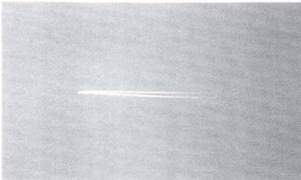
Figure 1. Photograph of a typical “short contrail,” i.e., a quickly evaporating contrail observed behind a light two-engine aircraft.
